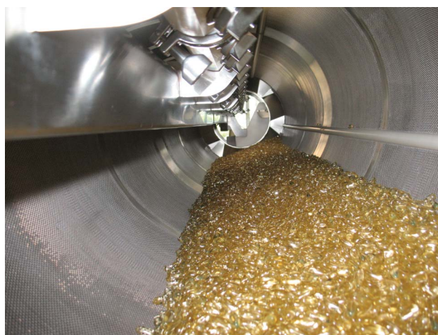
Figure 5. View of continuous coating pan loaded with 95 kg of soft gelatin capsules.
