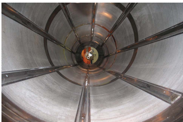
Figure 1. Interior view of coating chamber with the spray manifolds removed.
